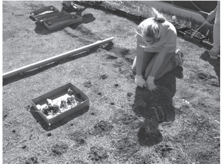
Atop the Pioneers Park Nature Center green roof, Kelsay Latshaw, a UCARE (Undergraduate Creative Activities and Research Experiences) worker and Landscape Architecture major, plants one of several treatment plots with native grasses and forbs.
