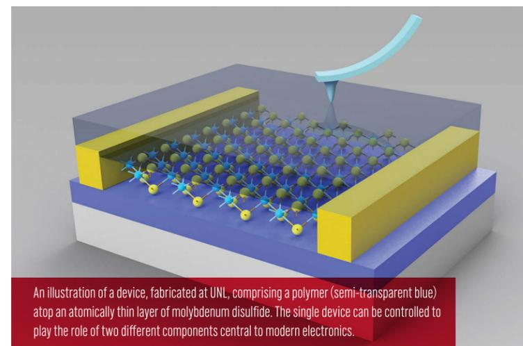
An illustration of a device, fabricated at UNL, comprising a polymer (semi-transparent blue) atop an atomically thin layer of molybdenum disulfide. The single device can be controlled to play the role of two different components central to modern electronics.
