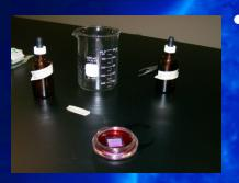
Soak the slide (face down) for 10 minutes in this liquid to stain the slide to a deep red-purple color. If the slide is not uniformly stained, then put it back in the liquid for 5 more minutes.
