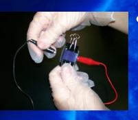
Connect a multimeter using an alligator clip to each plate (the negative electrode is the TiO<sub>2</sub> coated glass and the positive electrode is the carbon coated glass).
