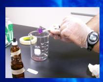
Wash the slide first with distilled water then ethanol and gently blot it dry with a tissue.
