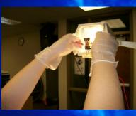
Make sure the light is shining through the TiO<sub>2</sub> coated glass first.
