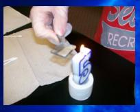
Pass the other piece of tin oxide glass, conducting side down, through a candle flame to coat the conducting side with carbon (soot).
